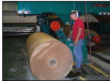
Manual or Automatic roll loading.
